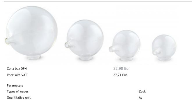
Hollow glass bulb with a narrow tube leading out for demonstrating acoustic resonance. The fundamental oscillation is generated by blowing into the opening or banging on the outside of the bulb.
