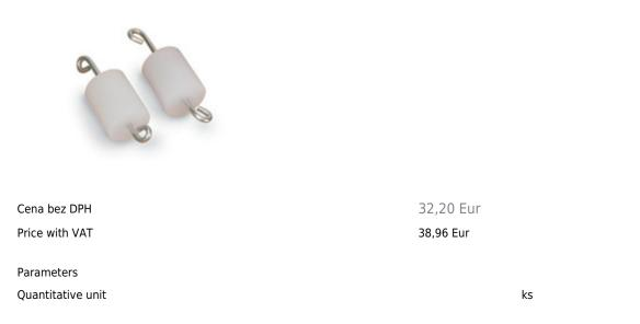
Two identical plastic cylinders with a density close to that of water. If the first is immersed in hot water, it will initially sink but will then float up to the surface after a short time. If the second one is then put into ice-cold water, it will initially float but will then sink to the bottom. The reason for this is that the density of the plastic changes more than that of the water when it is heated or cooled.
