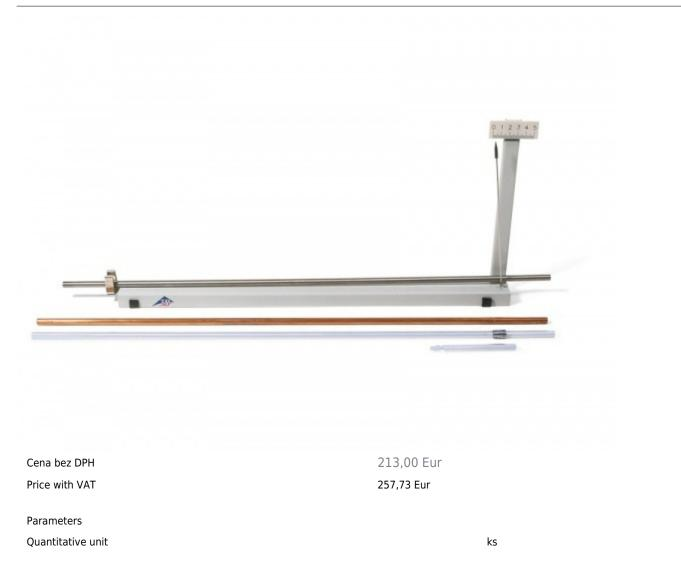
A device for measuring the thermal expansion of solids in dependence on length and material. The scope of delivery includes three sample tubes (steel, brass and glass) which are heated by passing water vapor through them. Consists of a base strip with a fixed bearing, pilot bearing, pointer and projectable scale.
