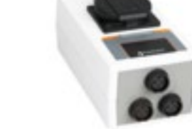
Switchbox Connect up to three rotary evaporators to one vacuum pump If no vacuum is required or when the required vacuum has been reached, the pump is switched off automatically. Prevents excess energy consumption. For applications with different pressure settings, each evaporator must be equipped with vacuum valve and non-return valve. Delivery includes three non-return valves. Suitable only for Hei-VAP Control models Weight 0.6 kg, w/d/h 80×45×160 mm P/N 569-00400-00
