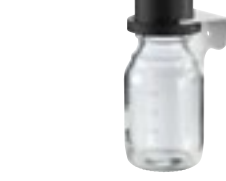
Woulff bottle For separating condensate to protect the valves of the vacuum pump, standard vacuum laboratory bottles can be used. Screw connection for easy emptying and cleaning, compatible with all Hei-VAP configurations, volume of 200 ml P/N 569-00071-00
