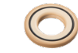
Vacuum seal PTFE/FFKM Special PTFE seal (with FFKM sealing ring), highest chemical resistance, long lifespan without abrasion, highest density, FDA-compliant P/N 23-30-01-06-70 Standard PTFE/FKM spare seal P/N 23-30-01-01-30
