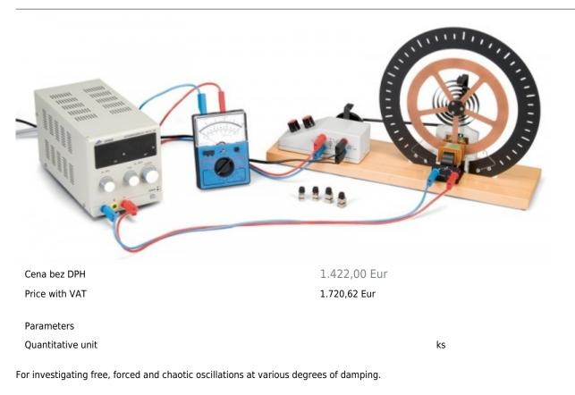
With slotted scale ring and pointers on resonator and exciter.
