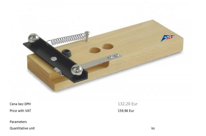
For demonstrating unimpeded superimposition of motions. A launching rail with returning spring is mounted on a wooden base. Two steel balls are used as test bodies. Upon triggering, one ball starts to fall downwards and simultaneously the other is launched horizontally. Both balls hit the ground at the same time. Two holes in the base plate are provided for storing the balls.
