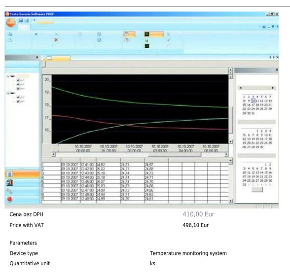
The testo Saveris monitoring system saves time thanks to automated measurement and offers centralised documentation as well as an alarm function. It guarantees the safety of your measurement data in production processes, during the storage of pharmaceutical products and in clean room air conditioning.
