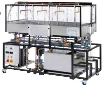
HM 141 Hydrographs after precipitation Correlations between precipitation and seepage; various drainage methods
