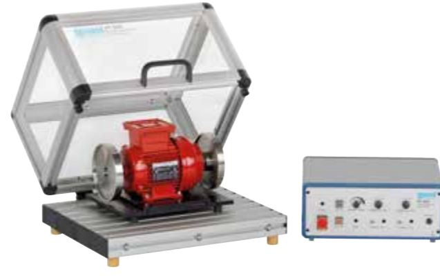
PT 502 Field balancing Measurement of imbalance vibrations
