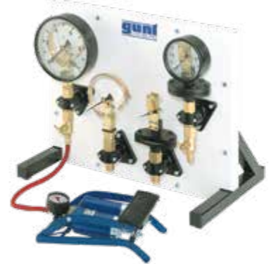
HM 700.16 Cutaway models: pressure gauges
