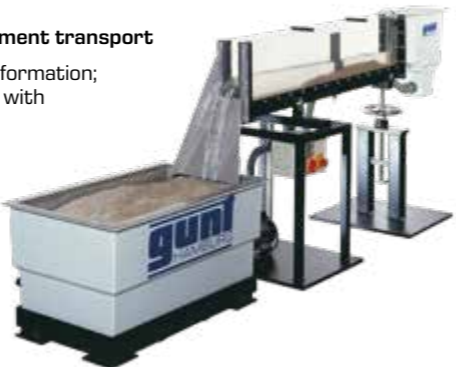
HM 144 Formation of river courses Compact experimental flume for modelling small river courses; inclination of the experimental flume adjustable
