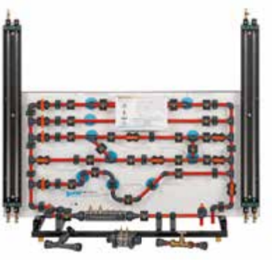
HM 150.11 Losses in a pipe system Influence of flow velocity on pressure loss Recommended for water supply: HM 150 Base module for experiments in fluid mechanics
