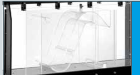
HM 162.36 Siphon weir
