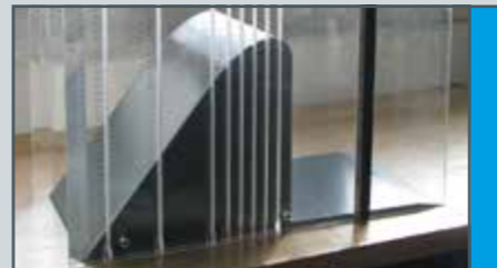
HM 162.34 Ogee-crested weir with pressure measurement
