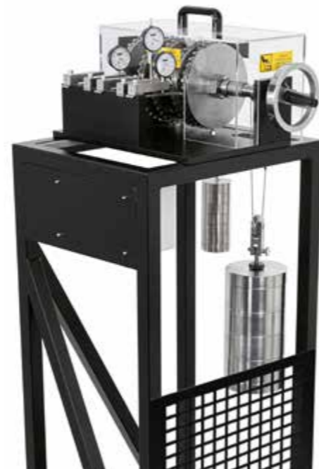
GL 212 Dynamic behaviour of multistage planetary gears Investigation of rotational dynamics of a two-stage epicyclic gear with three planetary gears each; four different transmissions adjustable
