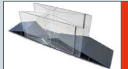
HM 162.55 Parshall flume
