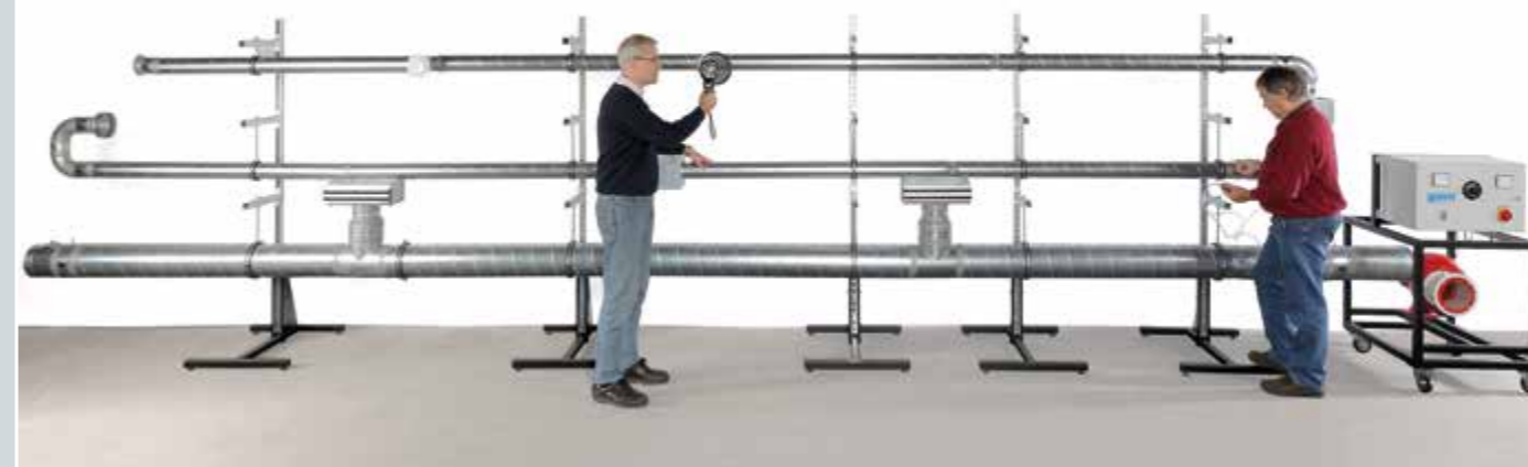
HL 710 Air duct systems Planning and setup of simple and complex air duct systems
