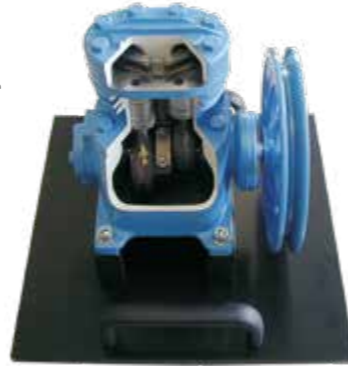
ET 499.03 Cutaway model: open refrigerant compressor, two-cylinder
