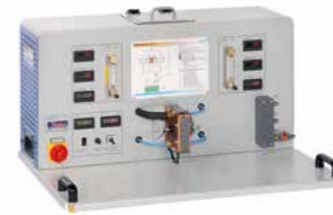
ET 360 Refrigeration circuit with propane
