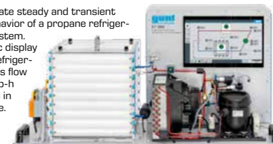
ET 360 Refrigeration circuit with propane
