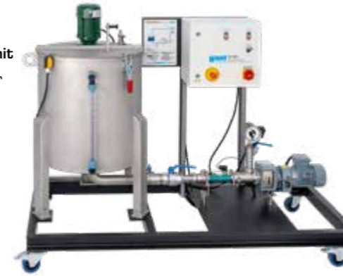
CE 579 Depth filtration Demonstration of depth filtration and backwashing of filters
