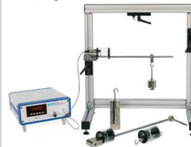
FL 100 Strain gauge training system Basic introduction to measurement with strain gauges for tension, bending and torsion
